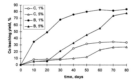
Fig. 2. The influence of pulp density (1%, 5%) on dynamics of chemical (C) and bacterial (B) leaching of cobalt from pentlandite.
