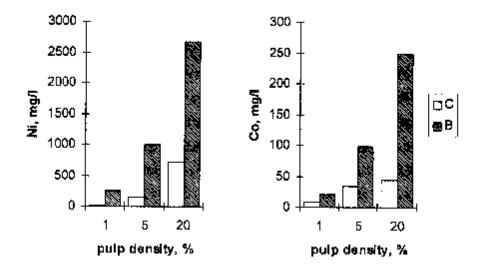
Fig. 3. The influence of pulp density on nickel and cobalt concentrations in the solutions obtained after chemical (C) and hacterial (B) leaching of penthandite.
