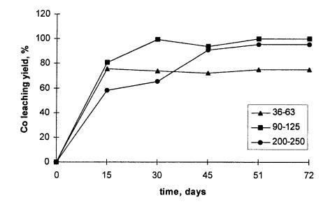
Fig. 5. The influence of particle size (36-63 μm, 90-125 μm, 200-250 μm) on cobalt bacterial leaching from pentlandite.
